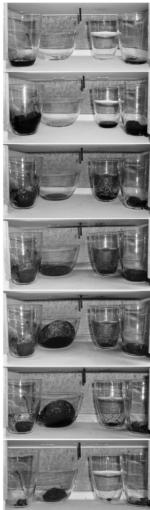
Fig. 2. Tracking the incineration of megestrol acetate, phthalazine derivative, azelaic acid and lactose (from the left) in the microwave muffle furnace at different temperatures (from the top to the bottom): room temperature, 103, 209, 301, 402, 502 and 599 °C. Temperature program: 40–500 °C in 3.5 h (hold for 1 min), afterwards to 600 °C in 8 min.
